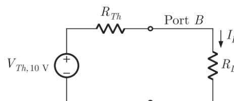
$$I_L = \frac{V_{Th,10V}}{R_{Th} + R_L}$$
