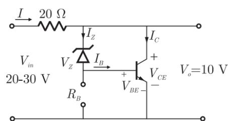
Maximum power will dissipate in Zener diode when current through it is maximum and it will occur at  $V_{in} = 30 \text{ V}$
