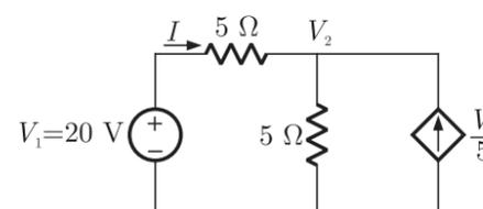
$$\frac{V_2}{5} + \frac{V_2 - V_1}{5} = \frac{V_1}{5}$$
