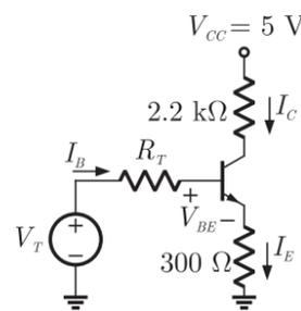
$$V_T = \frac{R_1}{R_1 + R_2} V_C = \frac{1}{4 + 1} \times 5 = 1 \text{ V}$$
