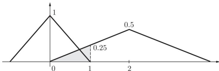
$$P(\text{error when bit 1 received}) = \frac{1}{2} \times 1 \times 0.25 = \frac{1}{8}$$
