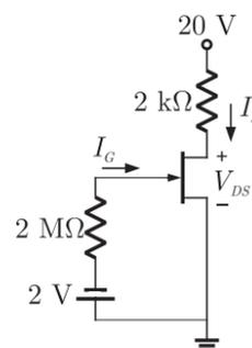
Since the FET has high input resistance, gate current can be neglect and we get  $V_{GS} = -2 \text{ V}$
