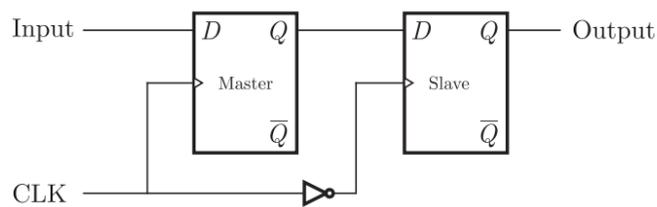
In the circuit we can see that output of flip-flop can be triggered only by transition of clock from 1 to 0 or when state of slave latch is affected.
