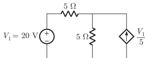
$$(A) \text{delivers } 80 \text{ W} \quad (B) \text{absorbs } 80 \text{ W}$$
