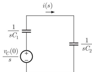
$$I(s) = \frac{v_c(0)/s}{\frac{1}{C_1 s} + \frac{1}{C_2 s}} = \frac{v_c(0)}{\frac{1}{C_1} + \frac{1}{C_2}}$$
