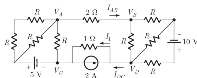
The total current in the resistor  $1 \Omega$  will be
