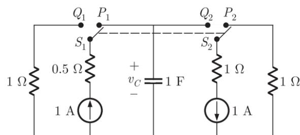
Assume that the capacitor has zero initial charge. Given that  $u(t)$  is a unit step function, the voltage  $v_c(t)$  across the capacitor is given by
