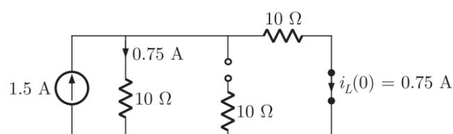
At  $t = 0$ , inductor current does not change simultaneously, So the circuit is
