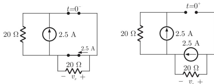
At  $t = 0^+$ ,  $i_L(0^+) = i_L(0^-) = 2.5 \text{ A}$  and all this current will pass through  $2 \Omega$  resistor. Thus
