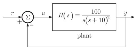
7.12 The gain margin of the system under closed loop unity negative feedback is
