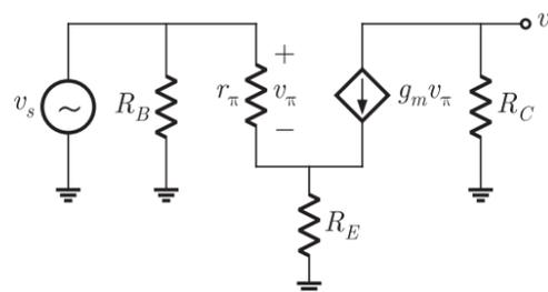
$$\text{Input impedance} \quad R_{in} = R_B || [r_\pi + (\beta + 1) R_E]$$
