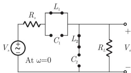
$$\frac{V_0}{V_s} = \frac{R_L}{R_L + R_s} \quad (\text{finite value})$$
