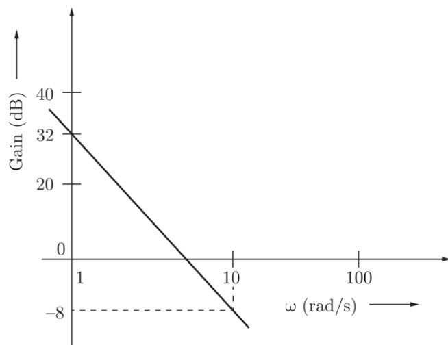
The gain ( $20 \log |G(s)|$ ) is 32 dB and -8 dB at 1 rad/s and 10 rad/s respectively. The phase is negative for all  $\omega$ . Then  $G(s)$  is
