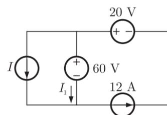
Since 60 V source is absorbing power. So, in 60 V source current flows from + to - ve direction
