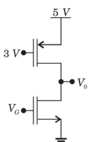
4.30 For small increase in  $V_G$  beyond 1V, which of the following gives the correct description of the region of operation of each MOSFET
