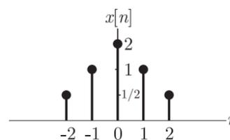
6.73 The sequence  $y(n) = \begin{cases} x(\frac{n}{2} - 1), & \text{For } n \text{ even} \\ 0, & \text{For } n \text{ odd} \end{cases}$  will be
