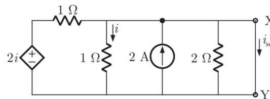
$$\text{Therefore } R_{th} = \frac{V_{th}}{i_{sc}} = \frac{4}{2} = 2 \Omega$$
