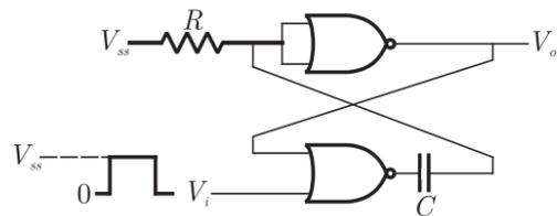
The circuit shown is monostable multivibrator as it requires an external triggering and it has one stable and one quasistable state.
