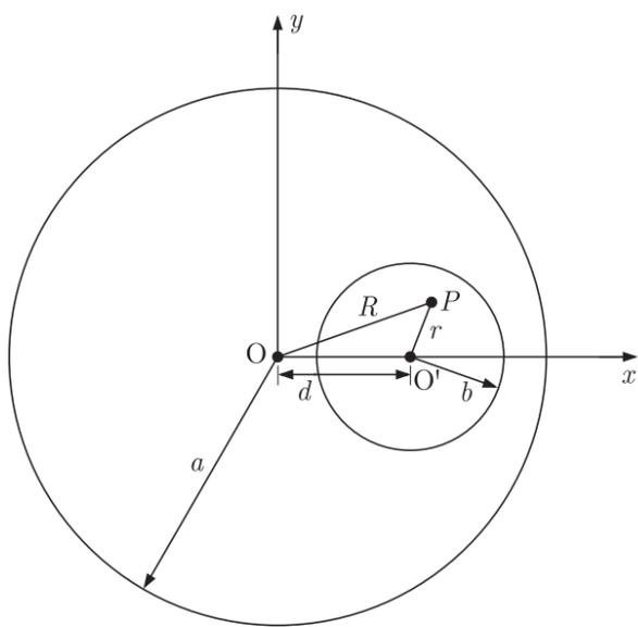
Since, the hole is drilled along the length of wire. So, it can be assumed that the drilled portion carries current density of  $-J$ . Now, for the wire without hole, magnetic field intensity at point  $P$  will be given as
