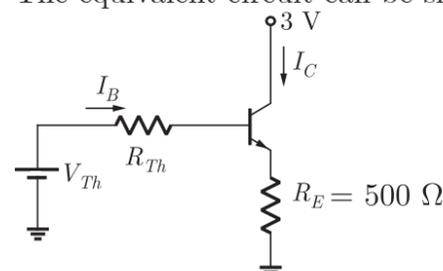
$$V_{Th} = V_{CC} \frac{R_2}{R_1 + R_2}$$
