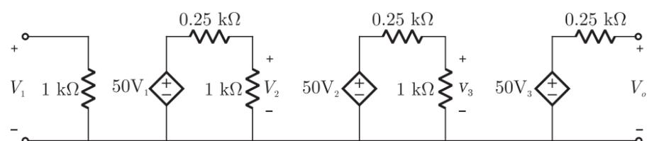
$$V_2 = \frac{1\text{k}}{1\text{k} + 0.25\text{k}} 50 V_1 = 40 V_1$$
