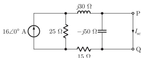
Using current divider rule the current  $I_{sc}$  is
