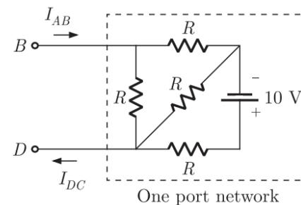
For a one port network current entering one terminal, equals the current leaving the second terminal. Thus the outgoing current from  $A$  to  $B$  will be equal to the incoming current from  $D$  to  $C$  as shown i.e.
