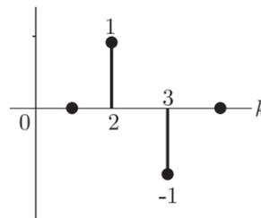
It has the finite magnitude values. So it is a finite impulse response filter. Thus  $S_2$  is true but it is not a low pass filter. So  $S_1$  is false.
