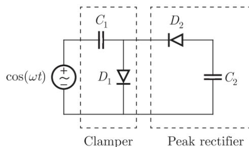
Clamper clamps the voltage to zero voltage, as shown
