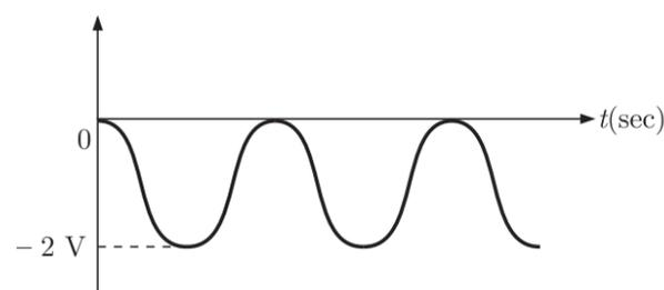
The peak rectifier adds +1 V to peak voltage, so overall peak voltage lowers down by -1 volt.
