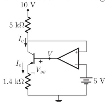
The voltage at non inverting terminal is 5 V because OP AMP is ideal and inverting terminal is at 5 V.
