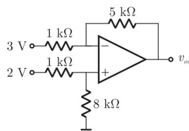
$$V_+ = \frac{8}{1+8}(3) = \frac{8}{3} \text{ k}\Omega$$
