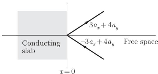
i.e. the reflected wave will be in direction  $3a_x + 4a_y$ . Thus, the electric field of the reflected wave will be.
