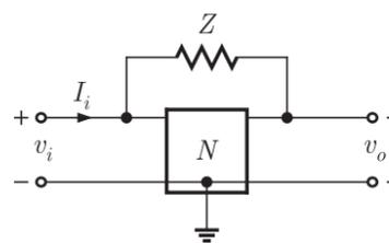
given input impedance is very large, so after connecting  $Z$  we have
