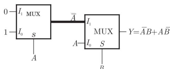
$$Y = \overline{B}I_0 + BI_1 = \overline{A}B + A\overline{B}$$
