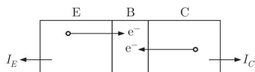
If both junction are forward biased and collector base junction is more forward biased then  $I_C$  will be flowing out wards (opposite direction to normal mode) the collector and it will be in reverse saturation mode.
