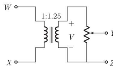
Since,  $\frac{V_{YZ}}{V} = 0.8$  (attenuation factor)
