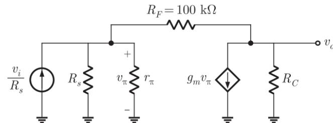
This is a shunt-shunt feedback amplifier.
