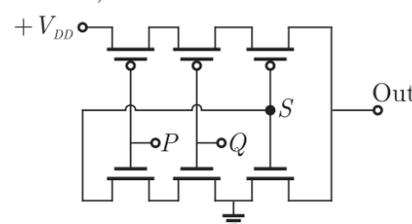
Since the lower MOSFETs are shorted to ground, node  $S$  is 0 only when input  $P$  and  $Q$  are 1. This is the function of AND gate.
