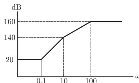
At  $\omega = 0.1$  change in slope is  $+60$  dB  $\rightarrow$  3 zeroes at  $\omega = 0.1$
