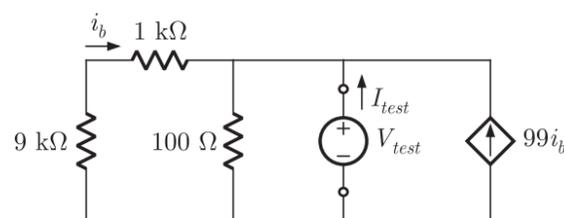
$$Z_{Th} = \frac{V_{test}}{I_{test}}$$
