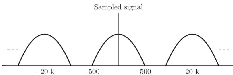
When sampled signal is passed through a *LP* filter of *BW* 1 kHz, only  $m(t)$  will remain.
