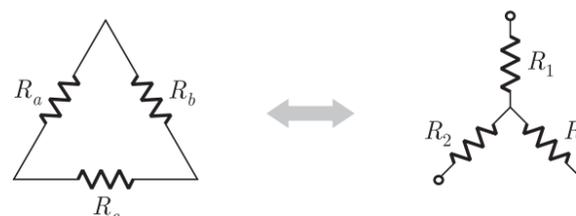
Thus  $R_1 = \frac{R_a R_b}{R_a + R_b + R_c} = \frac{6 \cdot 6}{6 + 6 + 6} = 2 \Omega$
