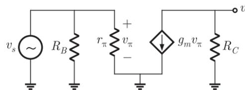
$$\text{Input impedance} \quad R_i = R_B || r_\pi$$
