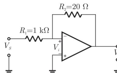
Let  $V$  be the voltage of inverting terminal, since non inverting terminal a at ground, the output voltage is
