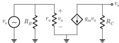
Input impedance  $R_i = R_B || r_\pi$
