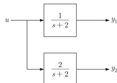
A state space model of the above system in terms of the state vector  $\underline{x}$  and the output vector  $\underline{y} = [y_1 \ y_2]^T$  is
