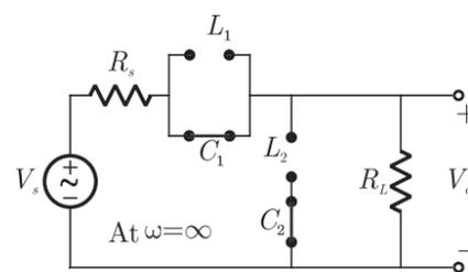
$$\frac{V_0}{V_s} = \frac{R_L}{R_L + R_s} \quad (\text{finite value})$$
