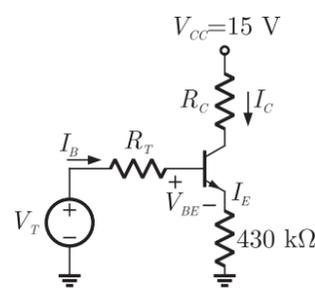
$$V_T = \frac{R_1}{R_1 + R_2} V_C = \frac{5}{10 + 5} \times 15 = 5 \text{ V}$$
