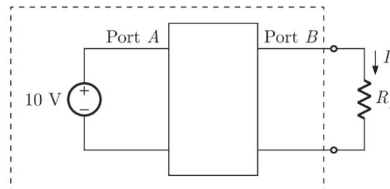
Now, we obtain Thevenin equivalent for the circuit seen at load terminal, let Thevenin voltage is  $V_{Th,10V}$  with  $10 \text{ V}$  applied at port  $A$  and Thevenin resistance is  $R_{Th}$ .
