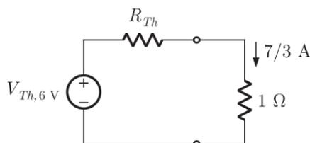
$$V_{Th,6V} = R_{Th} \times \frac{7}{3} + 1 \times \frac{7}{3} = 2 \times \frac{7}{3} + \frac{7}{3} = 7 \text{ V}$$
