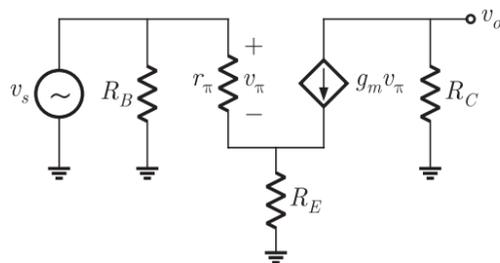
Input impedance  $R_{in} = R_B || [r_\pi + (\beta + 1) R_E]$
