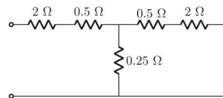
$$\text{Now} \quad z_{11} = \frac{V_1}{I_1} \Big|_{I_2=0} = 2 + 0.5 + 0.25 = 2.75$$
