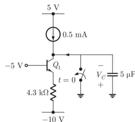
with time, the capacitor charges and voltage across collector changes from 0 towards negative.
