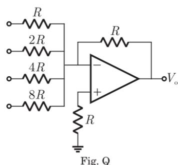
The input bits 0 and 1 are represented by 0 and 5 V respectively. The OP AMP is ideal, but all the resistance and the 5 v inputs have a tolerance of  $\pm 10\%$ . The specification (rounded to nearest multiple of 5%) for the tolerance of the DAC is
