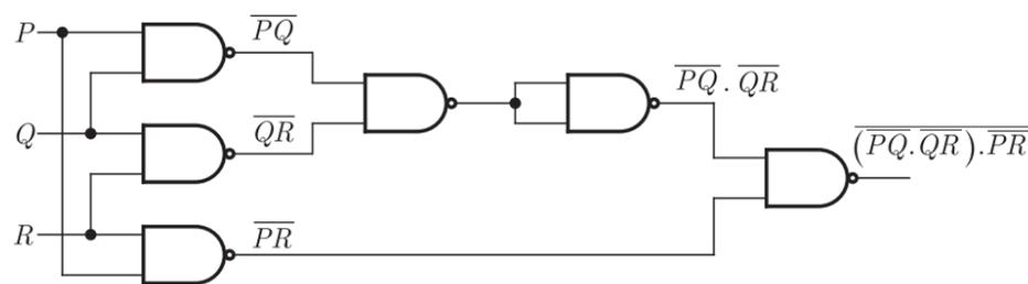
$$\begin{aligned} \overline{(\overline{PQ} \overline{QR}) \overline{PR}} &= \overline{(\overline{PQ + QR + PR})} \\ &= \overline{\overline{PQ + QR + PR}} \\ &= PQ + QR + PR \end{aligned}$$
