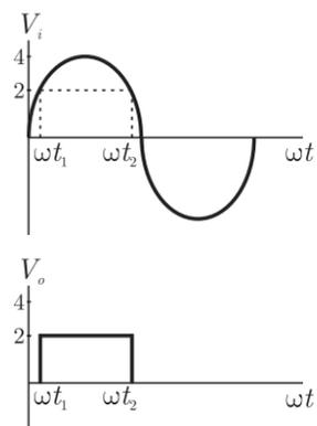
From fig, first crossover is at  $\omega t_1$  and second crossover is at  $\omega t_2$  where
