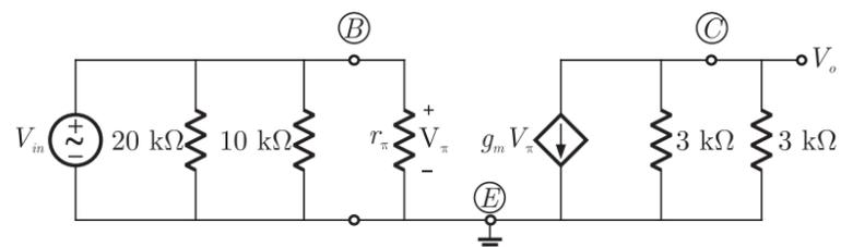
$$g_m = \frac{|I_C|}{V_T} = \frac{1\text{m}}{25\text{m}} = \frac{1}{25} \text{ A/V} \quad I_C \approx I_E$$
