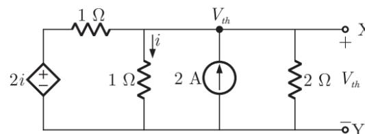
$$\frac{V_{th}}{2} + \frac{V_{th}}{1} + \frac{V_{th} - 2i}{1} = 2$$
