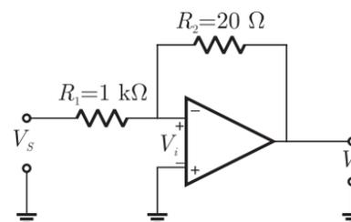
The closed-loop gain  $\frac{V_o}{V_s}$  is
