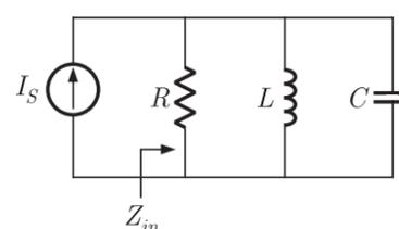
Input impedance  $Z_{in} = \frac{1}{\frac{1}{R} + \frac{1}{j\omega L} + j\omega C}$
