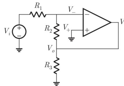
$$\text{So, } \frac{0 - V_i}{R_1} + \frac{0 - V_o}{R_2} = 0$$
