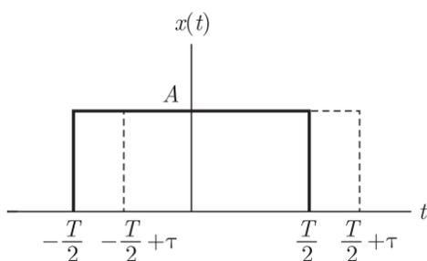
$$\begin{aligned} R_{xx}(\tau) &= \frac{1}{T} \int_{-T/2+\tau}^{T/2} A^2 dt \\ &= \frac{A^2}{T} \left[ \frac{T}{2} + \frac{T}{2} - \tau \right] = \frac{A^2}{T} \left[ \frac{T}{2} - \tau \right] \end{aligned}$$
