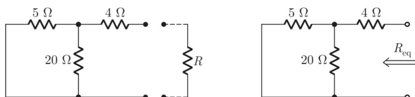
$$R_{eq} = 5\Omega \parallel 20\Omega + 4\Omega$$
