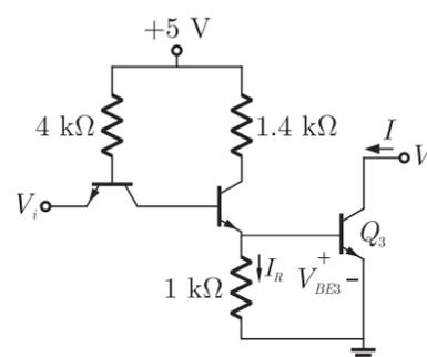
If output is at logic 0, then we have  $V_o = 0$  which signifies BJT  $Q_3$  is in saturation and applying KVL we have
