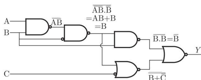
$$Y = \overline{B + (B + \overline{C})} = B(B + \overline{C}) = B$$
